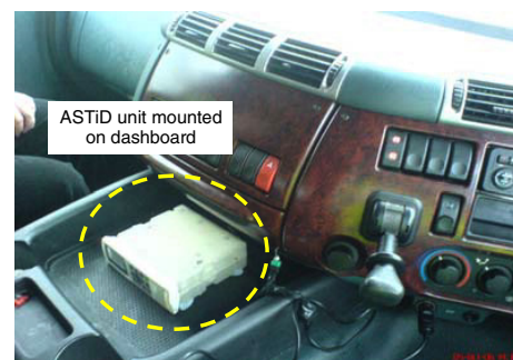
Figure 2. Shows the ASTiD system mounted on the dashboard of a vehicle.
